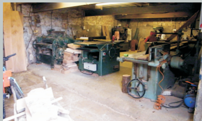
The workshop containing all the machinery needed to machine and finish timber
