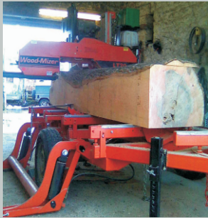
Wood-Mizer Bandsaw Mill, used to convert large logs
